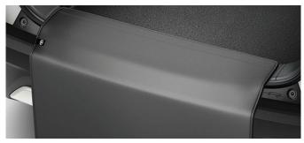
The rear bumper protection apron is fixed to the trunk deck with velcro. It protects the rear bumper when unfolded.
