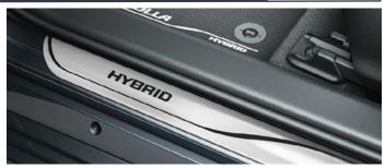
**ALUMINIUM SCUFF PLATES**Genuine scuff plates for the door sills create an immediate impression of style while also serving a very practical purpose of protecting the sill paintwork.
